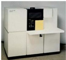
First computer-controlled ICP-MS
